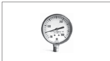
CENTER PORT COMPOUND GAUGE 30" Hg. - 150 PSI (2" FACE, 1/8"- NPT)
